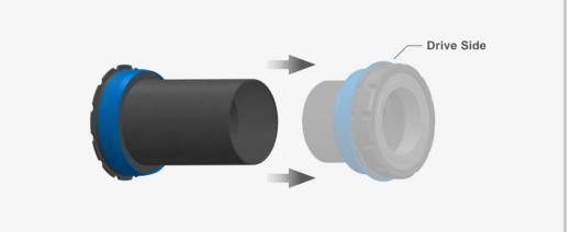
Gently position the non-drive side BB along with the non-drive side Snug Ring into the non-drive side of the BB shell. Using a dedicated BB installation tool, press the non-drive side BB into the BB shell of the frame until there is no gap between the BB and the frame.
