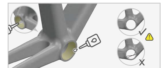
Remove the drive-side BB, which will be installed later.
