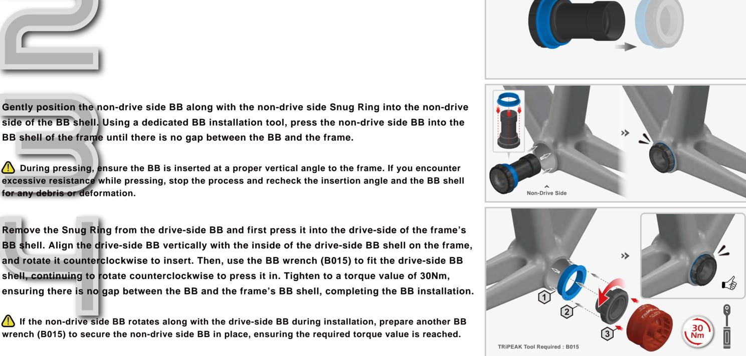
Installation of Crank's Adapter
